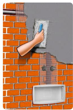
**CONMESH<sup>®</sup> LP/WP 1000 mm is very useful for Plaster / Gypsum Reinforcements, Waterproofing, Repair and Restorations, Concrete Grade Separations, Special Engineering requirements, Tensile Reinforcement etc.**
